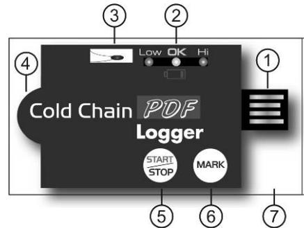
① USB2.0 plug & play connector. USB driver is not required.
